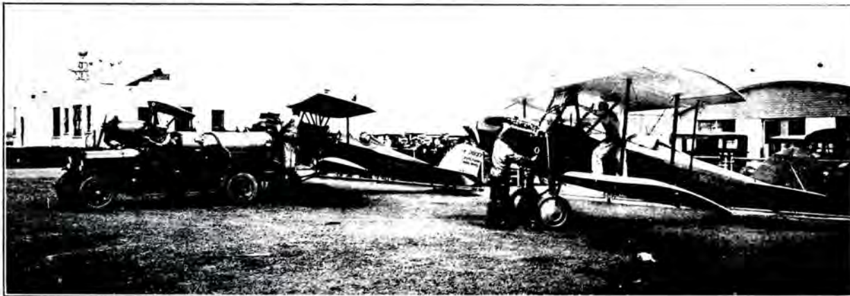
Fig. 10—Servicing Mail Plane from Airport Service Truck
